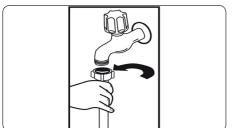
WARNING: Use the new water inlet hose supplied with your machine, do not use an old machine's hose.
